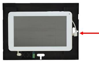
2. Screw the case back to the wall, bringing KeypadBus and power supply cables through the bottom or side entry.
