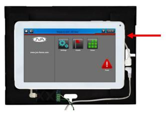
6. Replace the case front and secure with torx screws.
